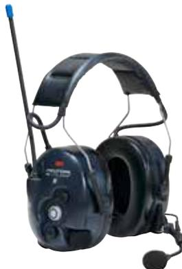
3M™ PELTOR™ LiteCom Communication Headsets have a communication radio built into a highly attenuating ear protection. In the WS headset, there is also a **Bluetooth®** link for connecting the headset to a mobile phone or another audio device with **Bluetooth®** functionality. Stereo microphones pick up the ambient sound which is reproduced inside the shells, while a level dependent surround sound function is effectively limiting impulse sounds to avoid hearing damage.
