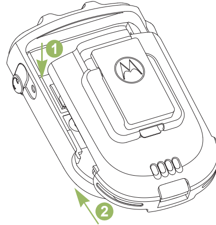
Figure 2.2: Attaching the battery into the WRSM
